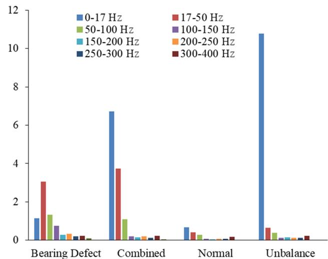
Fig. 8. Energy bands corresponding with the condition of the machinery.
