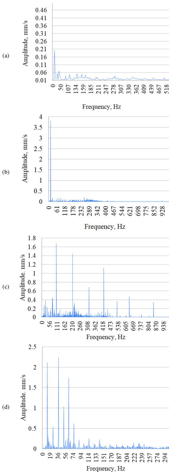
Fig. 5. Different machinery conditions. (a) Normal, (b) unbalanced, (c) bearing defect, (d) combined effect of unbalanced and bearing defect.
