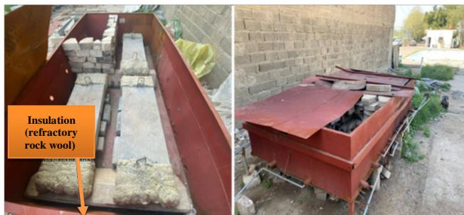
Fig. 5. Setup of the furnace and specimens.
