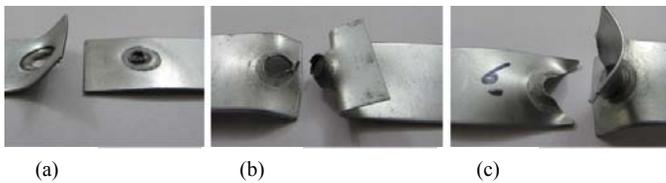
Fig. 13. Types of fractures in the tension-shear test
