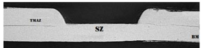
Fig. 4. Macro graphic FSSW joint for Galvanized BH plate
