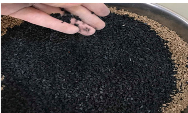
Fig. 1. The tire shreds used in this study.
