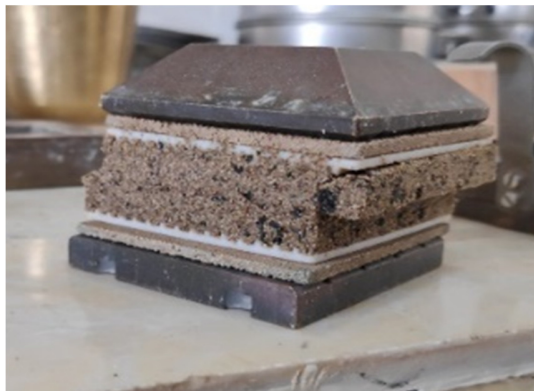
Fig. 3. The specimen of direct shear stress test.
