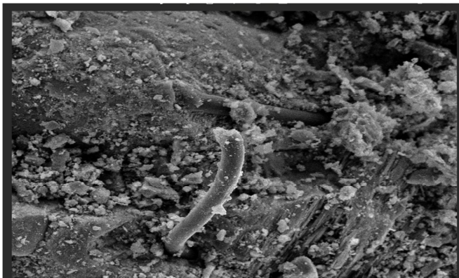
Fig. 13. The bond between PVA fibers and the matrix.
