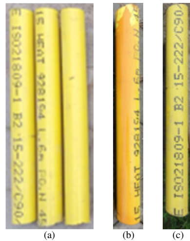
Fig. 3. Specimens of insulated pipe: (a) kept in water (b) or loam sand (c) for 72 hr.
