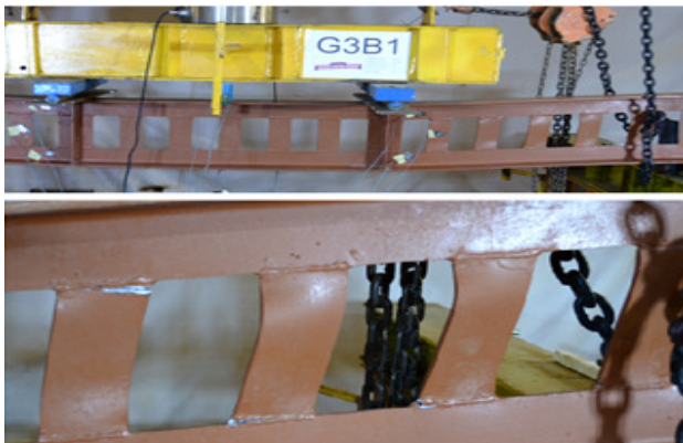
Fig. 18. Mode of failure for beam G3B1.
