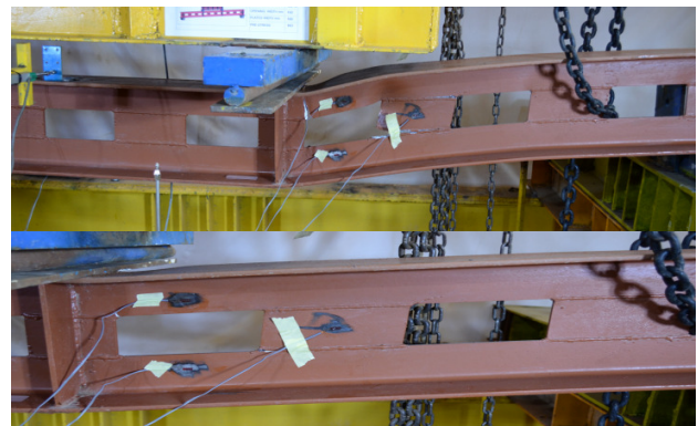
Fig. 17. Mode of failure for beam G2B2.
