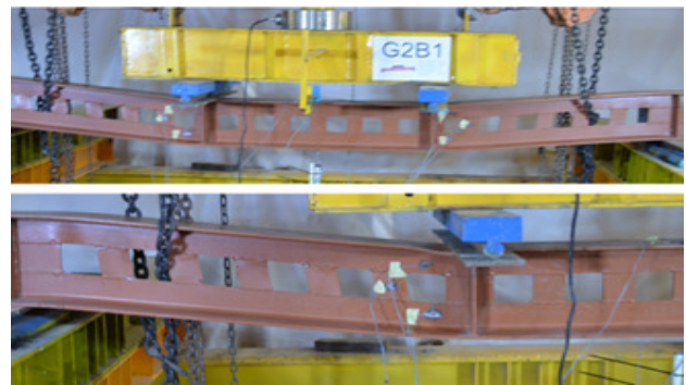
Fig. 16. Mode of failure for beam G2B1.
