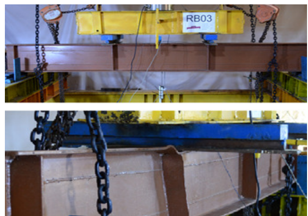
Fig. 12. Mode of failure for beam RB03.
