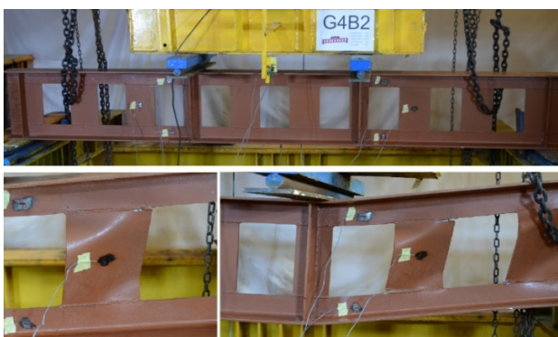
Fig. 21. Mode of failure for beam G4B2.
