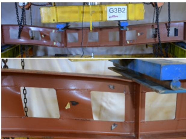
Fig. 19. Mode of failure for beam G3B2.
