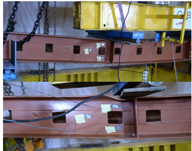
Fig. 15. Mode of failure for beam G1B2.
