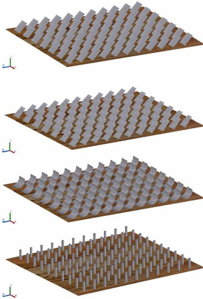
Fig. 1. Fin types (rectangular, trapezoidal, curved, and pin)
