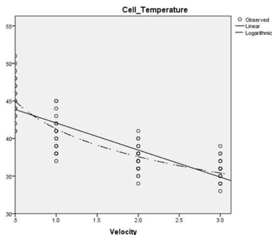
Fig. 2. The velocity magnitude and cell temperature diagram for the linear and logarithmic models
