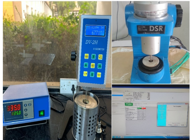
Fig. 3. Asphalt cement tests.
