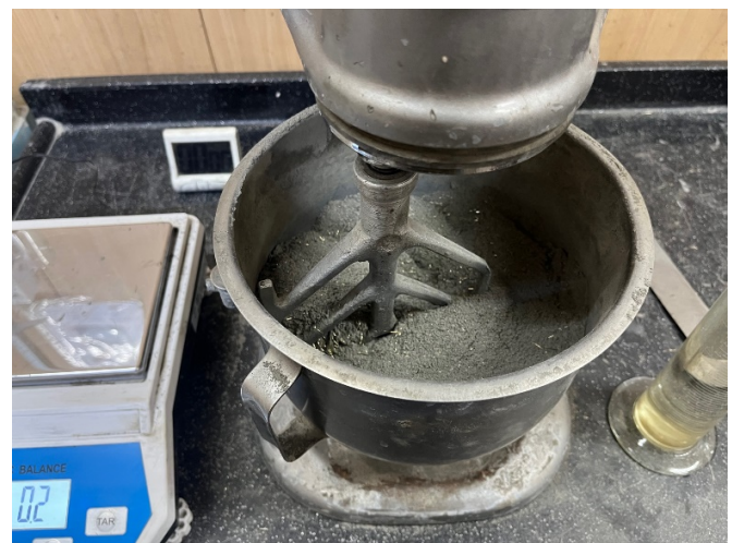
Fig. 1. Blending the ECC contents with a mechanical mixer.
