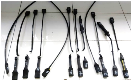
Fig. 6. PE100 SDR 11 samples after the tensile test.
