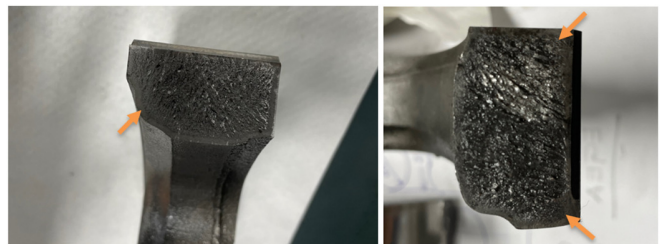
Fig. 10. Leg G (left) and Leg H (right) – arrows show the crack nucleation spots.
