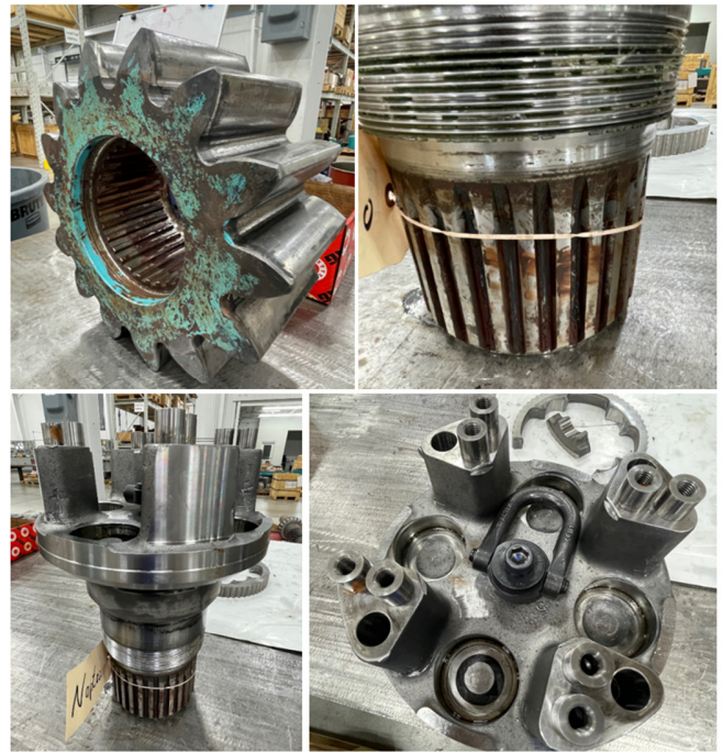
Fig. 2. Output gear, shaft spline with its upper base.
