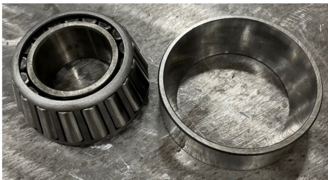
Fig. 12. Bearing that drives the cycloidal disc.
