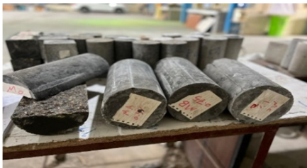
Fig. 5. Failure mode of concrete cylinders under splitting strength.
