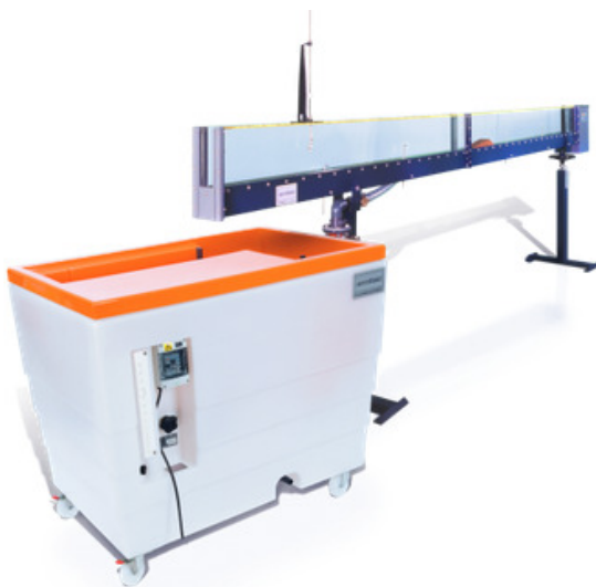
Fig. 2. The flume and hydraulic bench layout.
