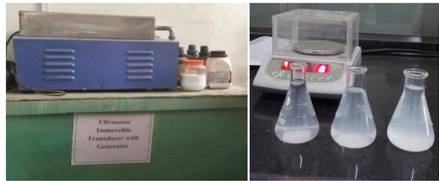
Fig. 3. The ultrasonic immersible transducer with generator and nanofluid samples.
