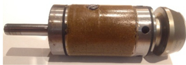
Fig. 4. Tested rotor casing with a rotor bearing inside.
