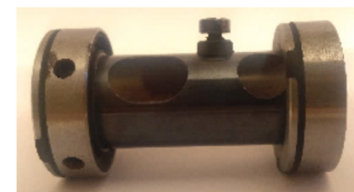
Fig. 1. Housing unit, its parts, and acoustic emission sensor.
