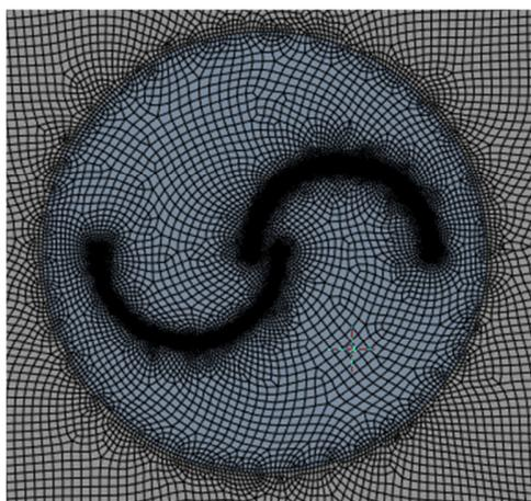
Fig. 3. Rotor's domain mesh.
