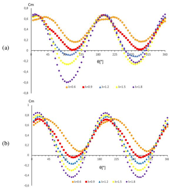
Fig. 5. The torque coefficient variation for the last complete revolution: (a) baseline, (b) optimized geometry.
