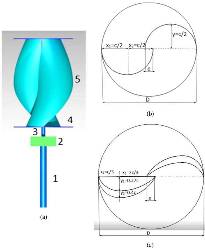
Fig. 1. Savonius 3D model, (b) baseline cross section, (c) optimized geometry cross section.
