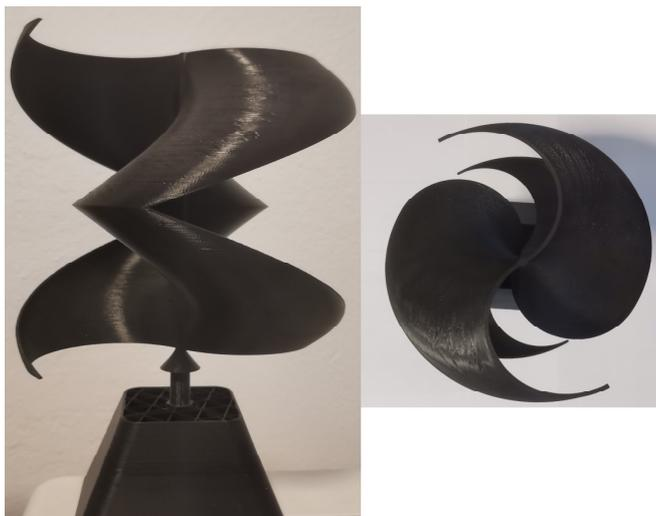
Fig. 8. 3D PLA print of the Savonius model.
