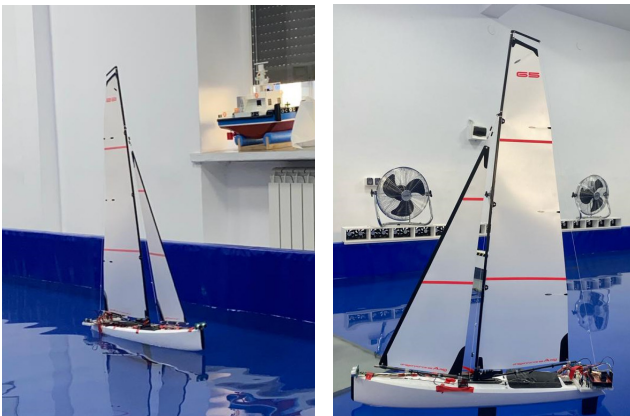
Fig. 9. Automated sail-propelled research boat in the test basin.
