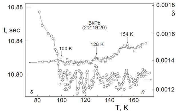
Fig. 6. Temperature dependence of the logarithmic damping decrement  $\delta$  and the period  $t$  of oscillation in the magnetic field of a ceramic sample of the nominal  $\text{Bi}_{1.7}\text{Pb}_{0.3}\text{Sr}_2\text{Ca}_{19}\text{Cu}_{20}\text{O}_y$ , obtained from precursors synthesized using solar technology.
