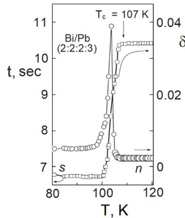
Fig. 5. Temperature dependence of the logarithmic damping decrement  $\delta$  and the period  $t$  of oscillation in the magnetic field of ceramic samples of the nominal  $\text{Bi}_{1.7}\text{Pb}_{0.3}\text{Sr}_2\text{Ca}_2\text{Cu}_3\text{O}_y$ , obtained from precursors synthesized using solar technology.
