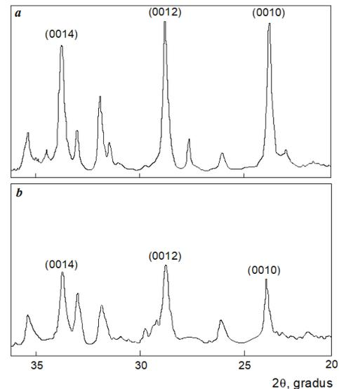
Fig. 1. Diffraction patterns of textured superconducting ceramics with the nominal composition  $\text{Bi}_{1.7}\text{Pb}_{0.3}\text{Sr}_2\text{Ca}_2\text{Cu}_3\text{O}_y$ , obtained from precursors synthesized in a solar oven: (a) at 817 °C for 65 hours, and (b) at 820 °C for 120 hours.
