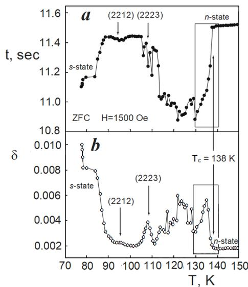
Fig. 4. Temperature dependence of the logarithmic damping decrement  $\delta$  and the period  $t$  of oscillation in the magnetic field of the ceramic sample of the nominal  $\text{Bi}_{1.7}\text{Pb}_{0.3}\text{Sr}_2\text{Ca}_3\text{Cu}_4\text{O}_y$ , obtained from precursor synthesized using solar technology (zero field-cooled ZFC-mode):  $s$ -state and  $n$ -state are superconducting and normal states, respectively.
