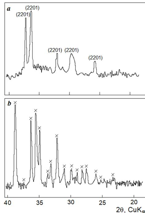
Fig. 2. Diffraction pattern of a precursor with the nominal composition  $\text{Bi}_{1.7}\text{Pb}_{0.3}\text{Sr}_2\text{Ca}_{19}\text{Cu}_{20}\text{O}_y$ , obtained by improved SFAQ-T: (a)-precursor (2201), (b) after annealing at 847 °C for 24 hours (x - phase 221920).
