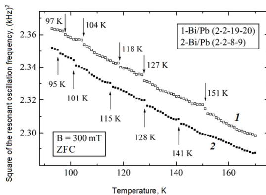
Fig. 7. Temperature dependence of the square of the natural frequencies of the multiphase samples (2-2-19-20) and (2-2-8-9) in a magnetic field of 300 mT.
