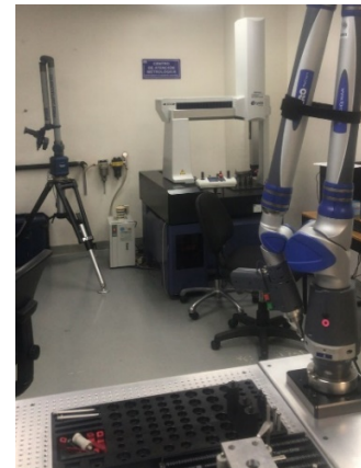
Fig. 1. Equipment of the metrology lab: articulated arms and CMM unit.
