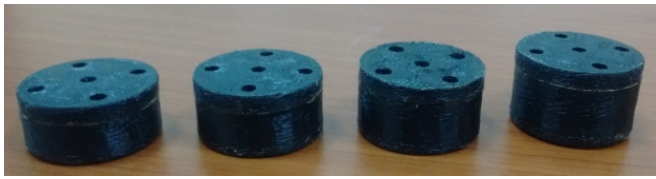
Fig. 4. Resonators designed for 2000 Hz – 2600 Hz.
