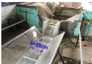
Fig. 2. The model from downstream to upstream (bed width 55 cm).
