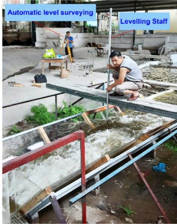
Fig. 4. Measuring water level data by the surveying equipment and the leveling staff (bed width b = 33.5 cm, Q = 136 l/s, and Fr_1 = 4.83 ).
