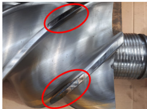
Fig. 6. Traces of rotors friction with the housing.
