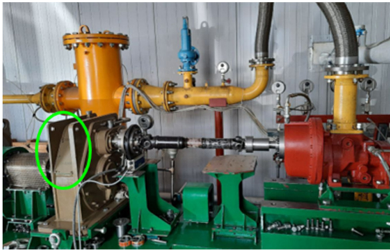
Fig. 3. Optimal screw mounting spot for the TEGs.
