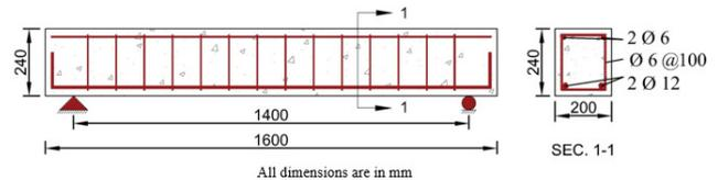
Fig. 2. Dimensions of the tested specimens and reinforcement details.
