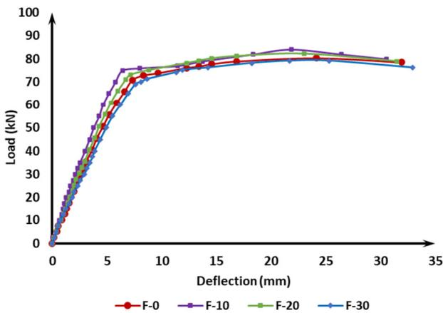
Fig. 13. Effect of LECA ratio on load-deflection behavior at mid-span.
