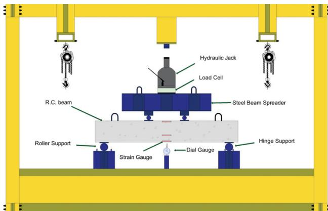
Fig. 4. Details of the test setup.
