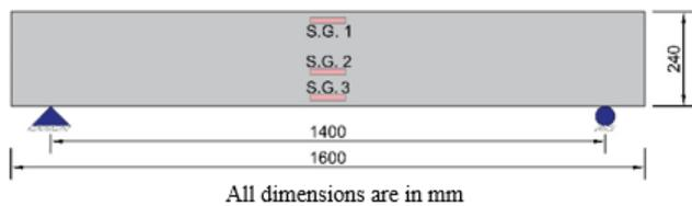
Fig. 14. Locations of the concrete strain gauges.
