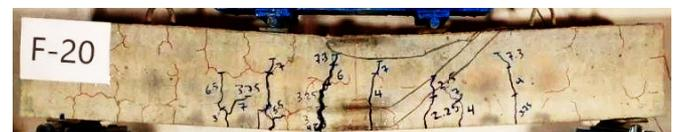
Fig. 11. Crack pattern for specimen F-20.
