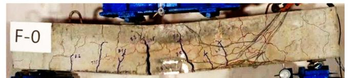
Fig. 9. Crack pattern for specimen F-0.
