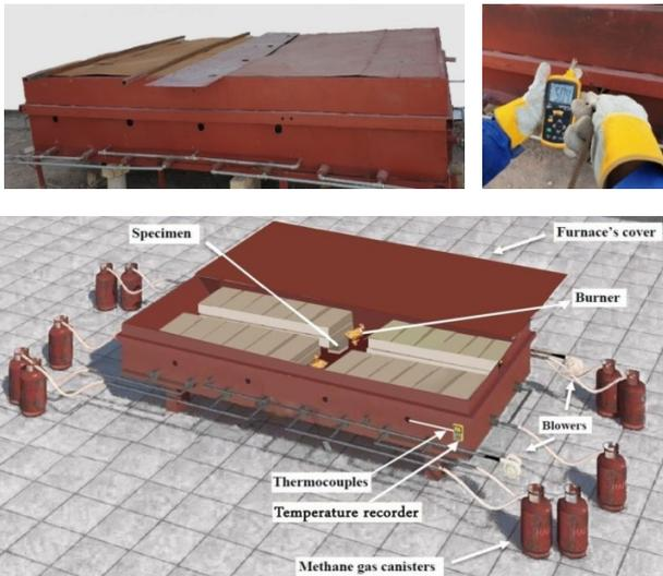
Fig. 3. Specimen burning procedure.
