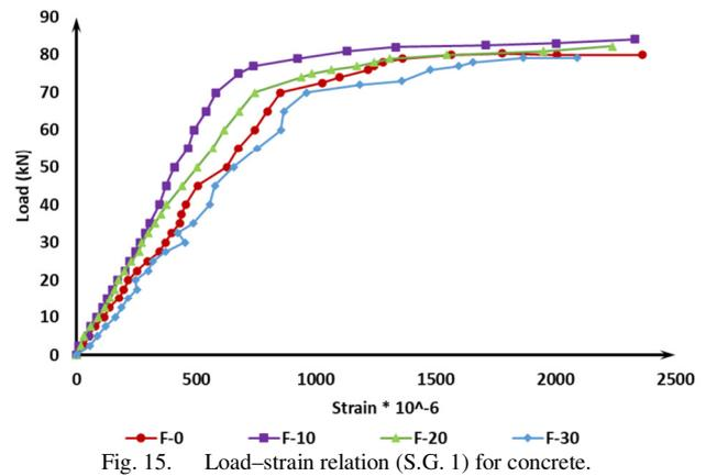
Fig. 15. Load-strain relation (S.G. 1) for concrete.
