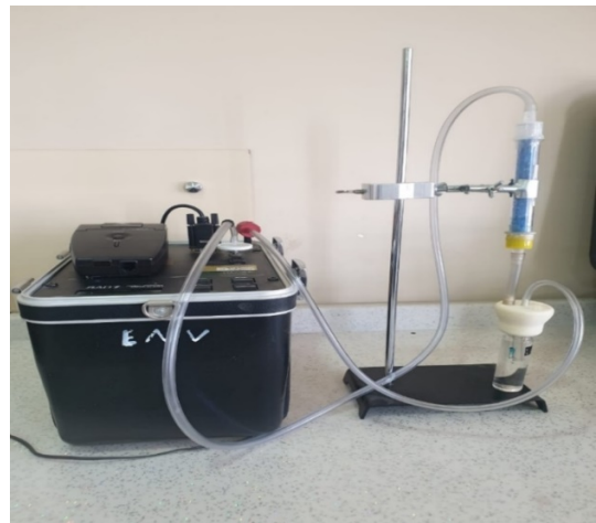
Fig. 2. Setup of the RAD7-Active Electronic Detector for measuring radon in water.
