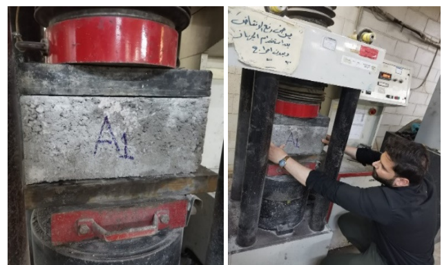
Fig. 6. Compressive strength test of concrete masonry units.
