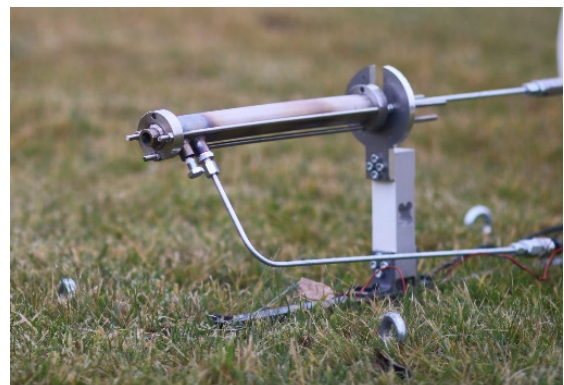
Fig. 20. Test bench with the integrated HRM after functioning.
