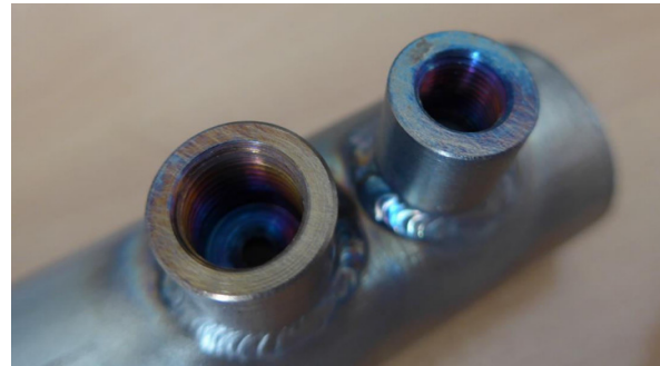
Fig. 12. Embossment welding for temperature and pressure measurement.
