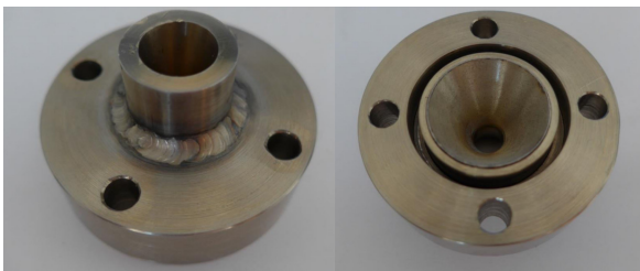
Fig. 10. Welding of the nozzle on the corresponding flange.
