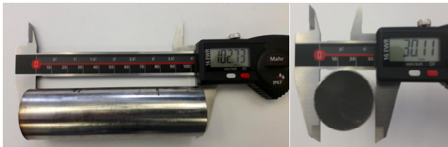
Fig. 4. Semifinished high temperature resistant steel (AISI 310S) bar before machining.
