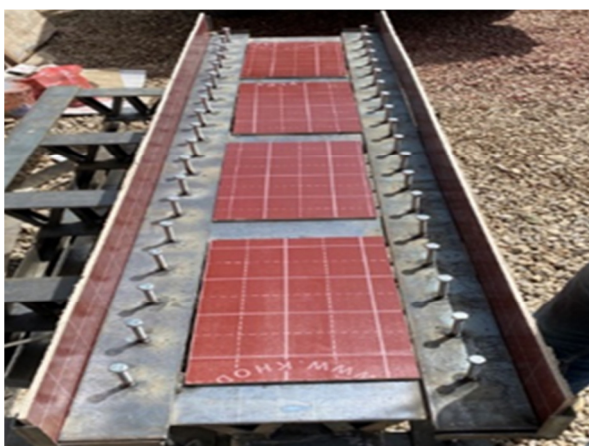
Fig. 2. Stud shear connector distribution.
