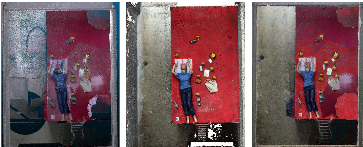
Fig. 7. Data output: 3D model point cloud of (a) TLS, (b) micro UAV, and (c) integrated point cloud.
