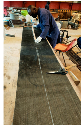
Fig. 2. Cutting the wrapping fabric into the desired sizes.
