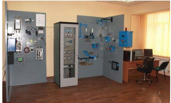
Fig. 6. Belt conveyor controlling hardware connected to the simulation model of whole mines factory.
