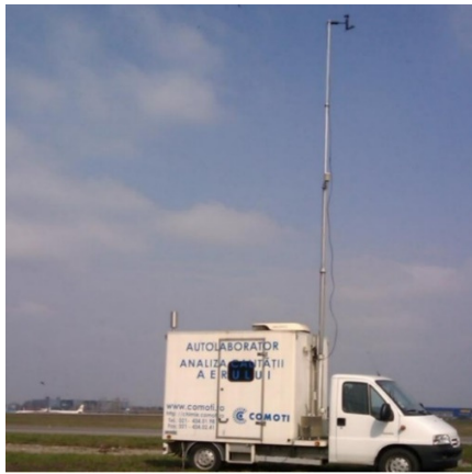
Fig. 3. The monitoring system of air pollutants.
