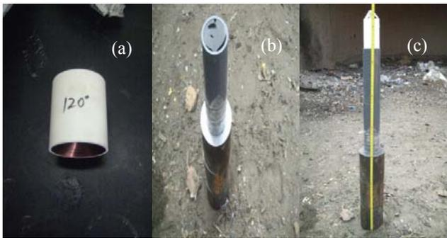
Fig. 8. (a) EFP change at rest (b) steel Target with 3CD water (c) setup for DOP Experiment
