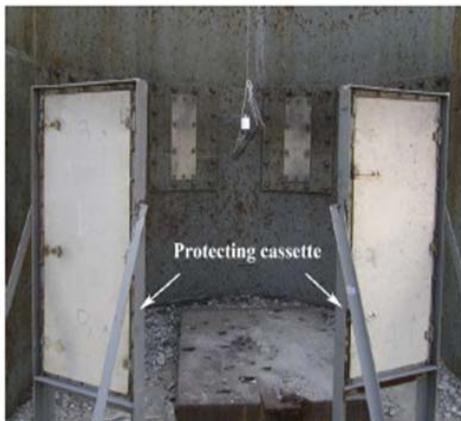
Fig. 5. Image of the Experimental test Setup with vertically hanging shaped charges.
