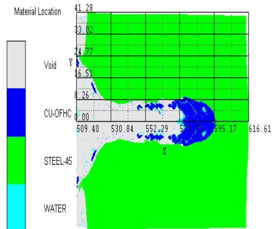
Fig. 3. Numerical simulation of the jet penetration against steel target.
