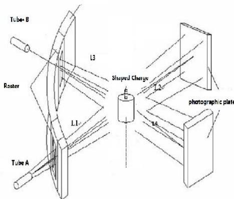
Fig. 6. Schematic of the test set up of 60 mm shaped charge in front of double flash X-Ray tube.
