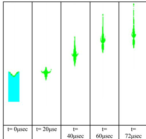
Fig. 2. Jet Formation at different time steps
