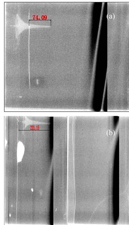
Fig. 7. (a) Jet Formation at 30 micro-Seconds (b) Jet Formation at 50 micro-Seconds
