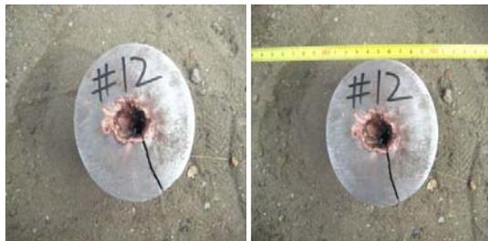
Fig. 9. EFP Jet Effect on the 45-steel Target
