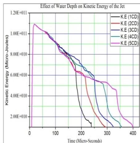
Fig. 4. Kinetic Energy behavior of the copper liner during jet formation and Penetration
