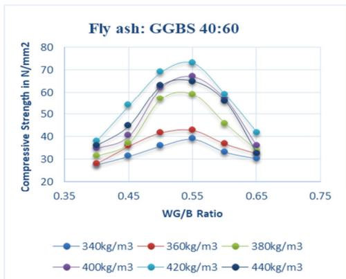
Fig. 3. Compressive strength of GPC for different WG/B F:G = 40:60.
