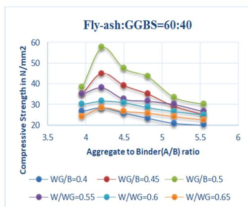
Fig. 6. Compressive strength of GPC for different AG/B to binder ratio and for F:G = 60:40.
