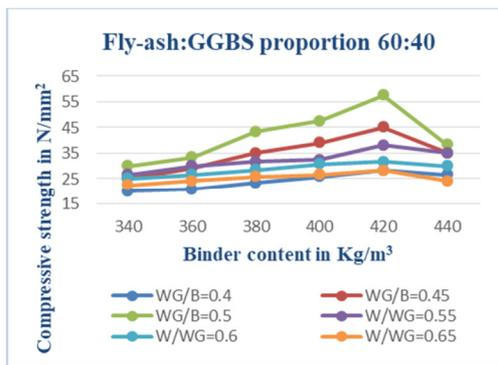
Fig. 8. Compressive strength of GPC for different binder content and for F:G = 60:40.
