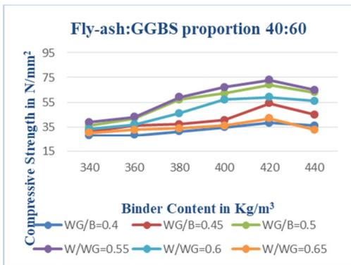
Fig. 9. Compressive strength of GPC for different binder content and for F:G = 40:60.
