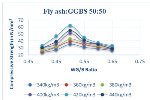
Fig. 2. Compressive strength of GPC for different WG/B and F:G = 50:50.
