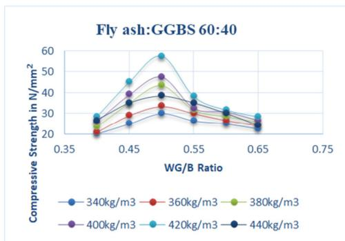
Fig. 1. Compressive strength of GPC for different WG/B and F:G = 60:40.
