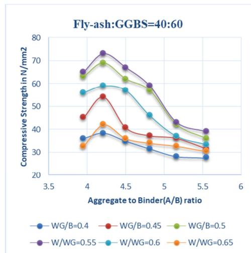
Fig. 4. Compressive strength of GPC for different AG/B to binder ratio and F:G = 40:60.
