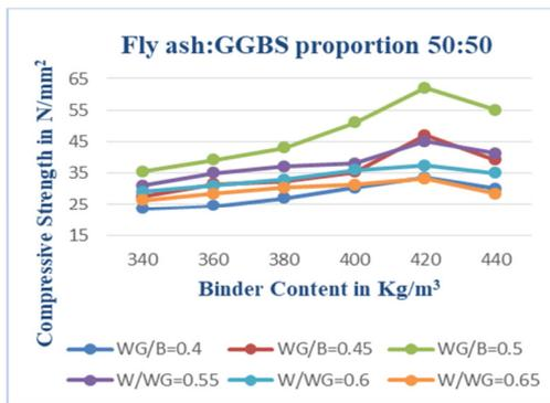
Fig. 7. Compressive strength of GPC for different binder content and for F:G = 50:50.
