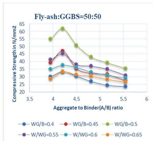
Fig. 5. Compressive strength of GPC for different AG/B to binder ratio and F:G = 50:50.
