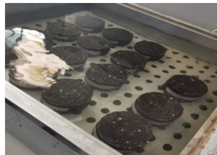
Fig. 1. Marshall test preparation.
