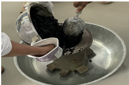
Fig. 4. Super-pave mold preparation.
