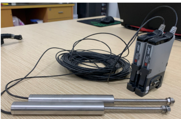
Fig. 6. LVDT sensors and cables.
