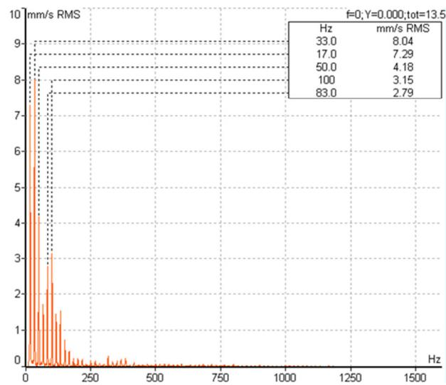
Fig. 5. Frequency spectrum of combined fault.
