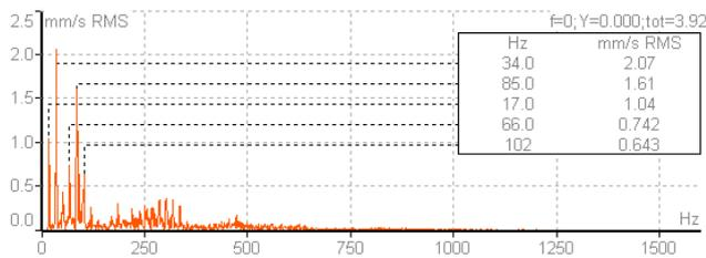
Fig. 4. Frequency spectrum of loosened fault.
