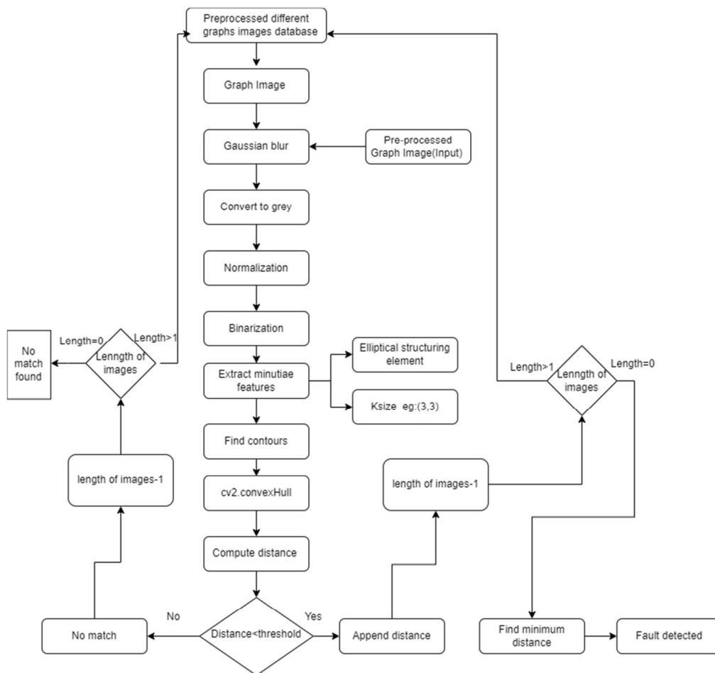
Fig. 6. Flow chart of the fault diagnostic system with the use of the Minutiae algorithm.
