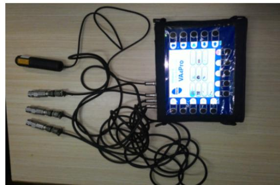
Fig. 2. The FFT analyzer.
