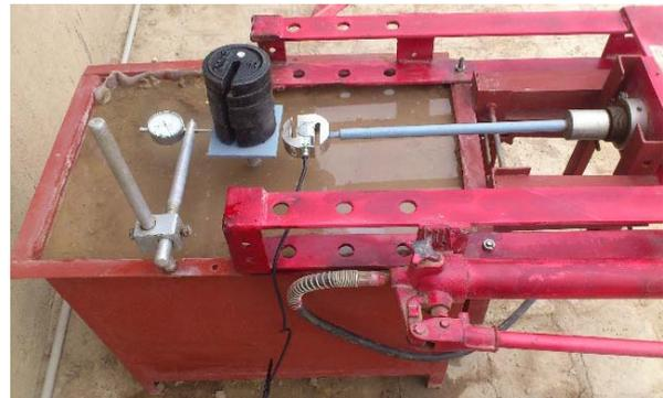
Fig. 2. Pile loading model-lateral displacement.
