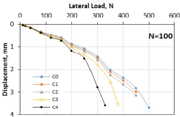
Fig. 12. Permanent lateral displacements versus lateral load at N = 100 cycles.
