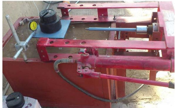
Fig. 1. Pile loading model-vertical displacement.
