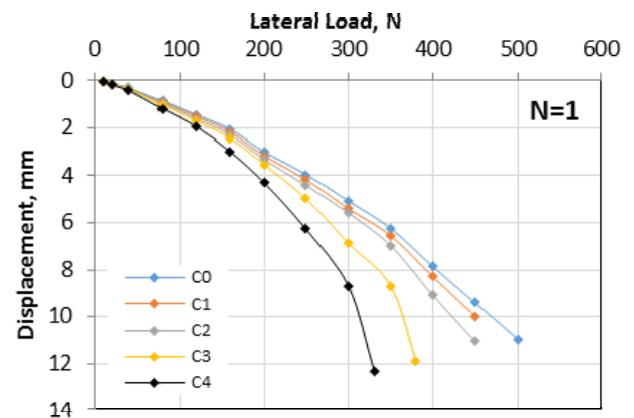
Fig. 5. Total lateral displacement versus lateral load at N = 1 cycle.
