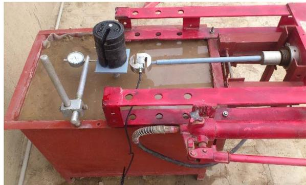
Fig. 2. Pile loading model-lateral displacement.
