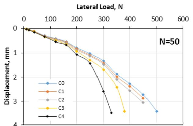
Fig. 11. Permanent lateral displacements versus lateral load at N = 50 cycles.
