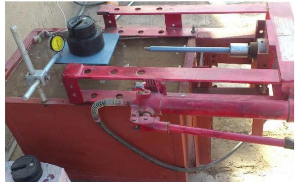
Fig. 1. Pile loading model-vertical displacement.
