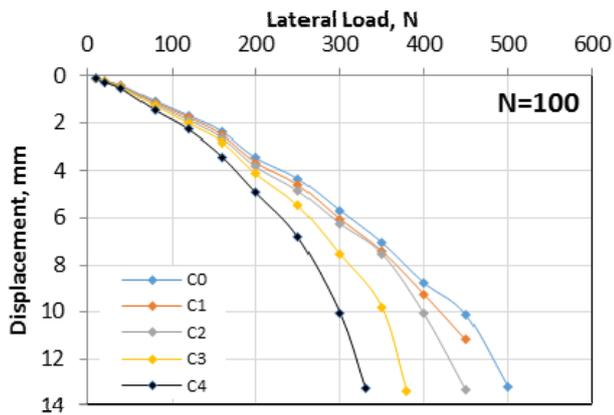
Fig. 8. Total lateral displacements versus lateral load at N = 100 cycles.
