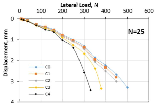
Fig. 10. Permanent lateral displacements versus lateral load at N = 25 cycles.
