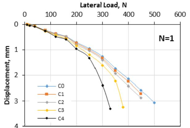
Fig. 9. Permanent lateral displacements versus lateral load at N = 1 cycle.
