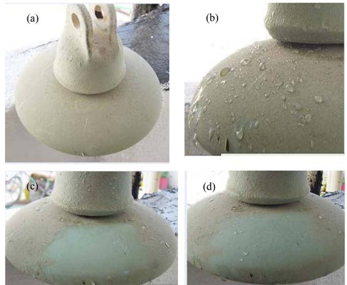
Fig. 2. SIR coated ceramic insulator
