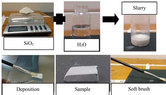
Fig. 5. Deposition of artificial pollution slurry on sample's surface
