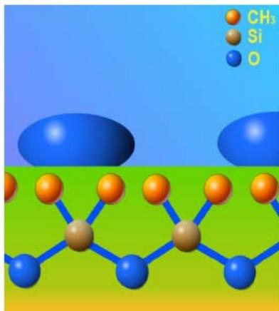
Fig. 1. Structure of silicone rubber.
