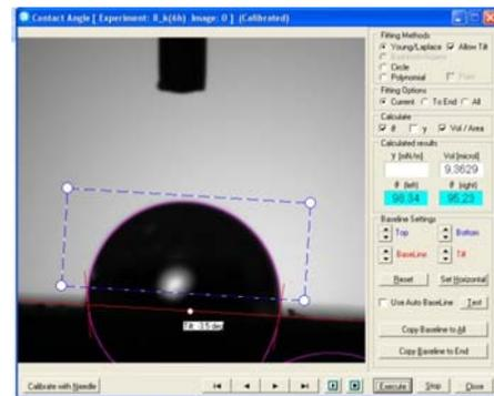
Fig. 6. Measure of contact angle
