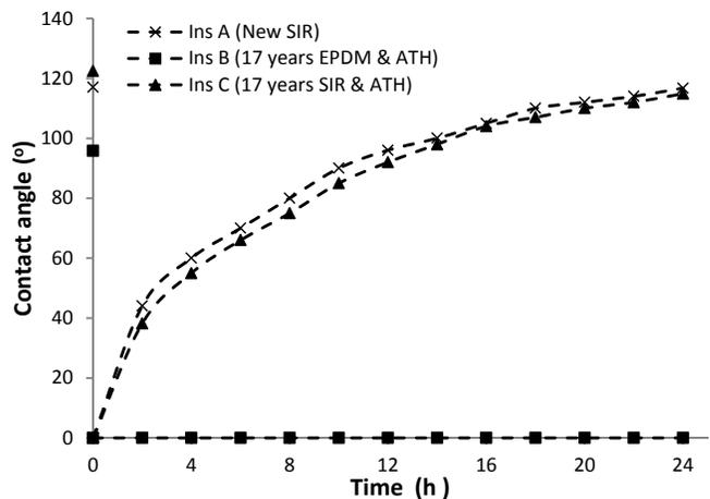
Fig. 7. Hydrophobicity transfer speed of insulators
