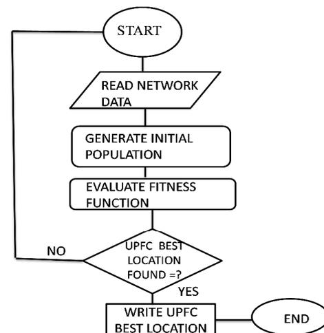
Fig. 4. Flowchart of the UPFC device optimal allocation process.
