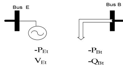
Fig. 3. UPFC static model.
