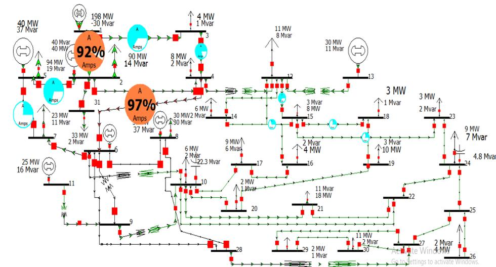
Fig. 7. UPFC located in line 2-6 (line 4-6 is shown in red despite 97% capacity).
