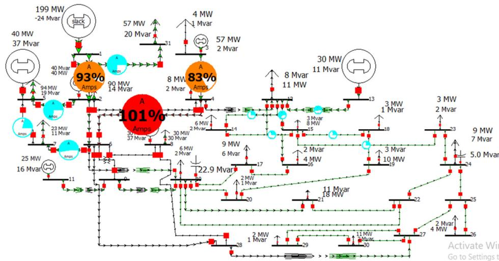
Fig. 6. UPFC located in line 1-3.
