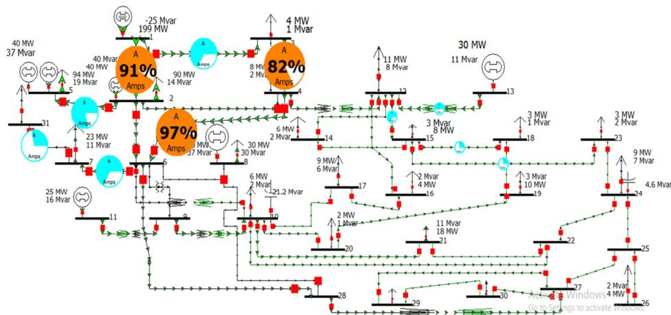
Fig. 8. UPFC located in line 5-7 (green indicates the flow in line 4-6 displays 97% loading).
