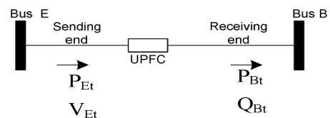
Fig. 2. UPFC power flow model.
