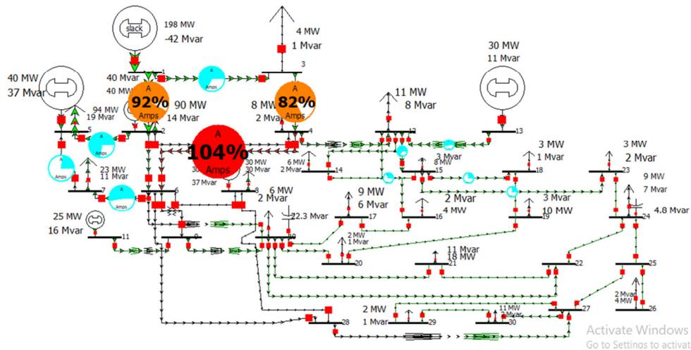
Fig. 5. System overload on line 4-6 of a modified IEEE 30 bus.
