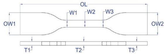
Fig. 2. Tensile test specimen - dimensional details.
