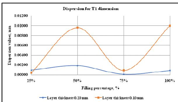
Fig. 5. The dispersion values for T1 dimension.
