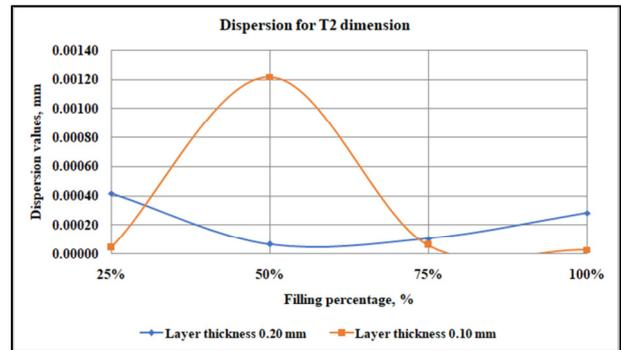
Fig. 6. The dispersion values for T2 dimension.
