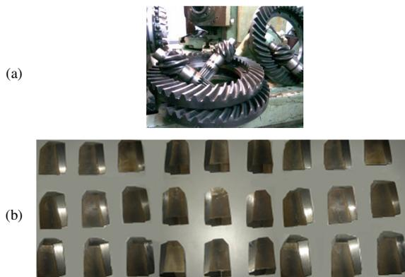
Fig. 1. Sample preparation: (a) Hypoid gear pairs after machining, (b) plasma nitriding samples cut from hypoid gears.
