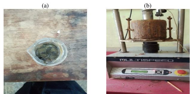
Fig. 1. Sample preparation and testing: (a) \beta -keratin extracted sample, (b) CBR test setup.
