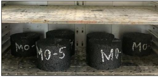
Fig. 1. Oven conditioning of asphalt mixtures.
