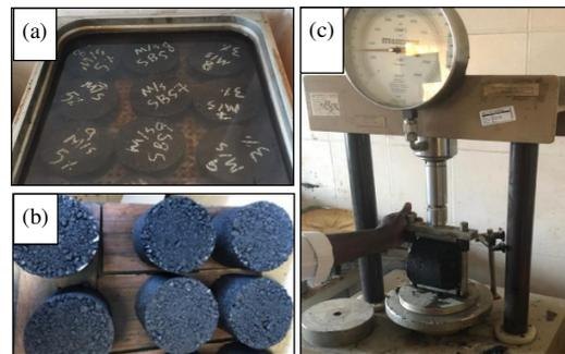
Fig. 4. a) Wet samples, (b) dry samples, (c) IDT testing.
