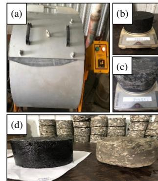
Fig. 3. Mixtures in the dynamic shear rheometer device (a) Abrasion drum, (b) CML before testing, (c) CML after testing, (d) CML before and after testing.
