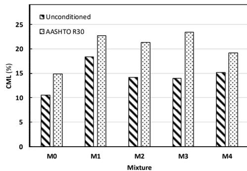
Fig. 8. Comparison of the unconditioned with AASHTO R30-conditioned CML.
