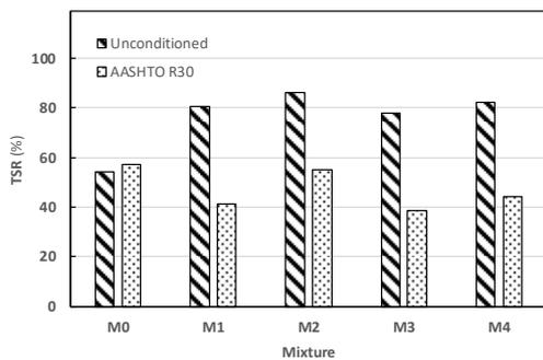
Fig. 7. Comparison of the Unconditioned with AASHTO R30 Conditioned TSR.
