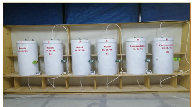
Fig. 2. Six bioreactor columns.
