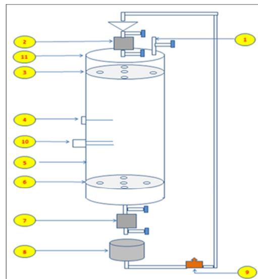
Fig. 1. Sketch of the anaerobic bioreactor. 1-Gas valve, 2-upper storage container for leachate recirculation, 3-upper perforated plate, 4-thermometer, 5-anaerobic biodegradation tank, 6-lower perforated plate, 7-leachate collection container, 8-extra leachate container, 9-pump, 10-pH and moisture content meter, 11-cover for waste feeding.
