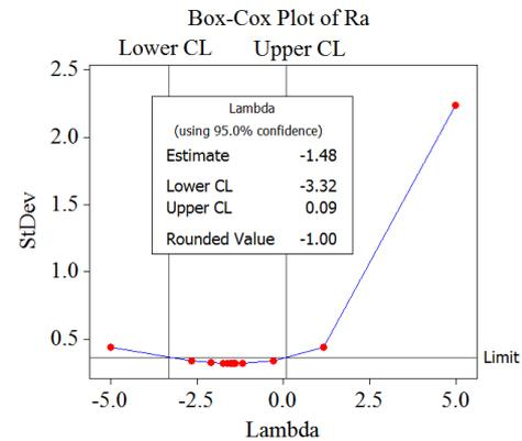
Fig. 2. Box-Cox transformation model of surface roughness
