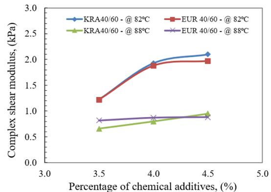
Fig. 4. Variations of complex shear modulus elastic portion with chemical additive percentage.
