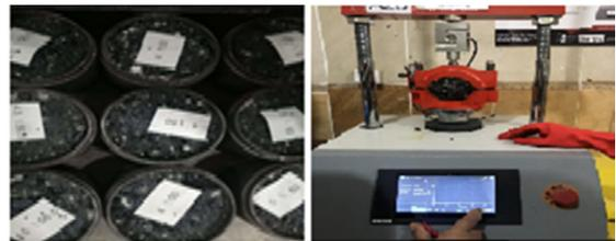
Fig. 2. Marshall specimens for three different additive percentages.
