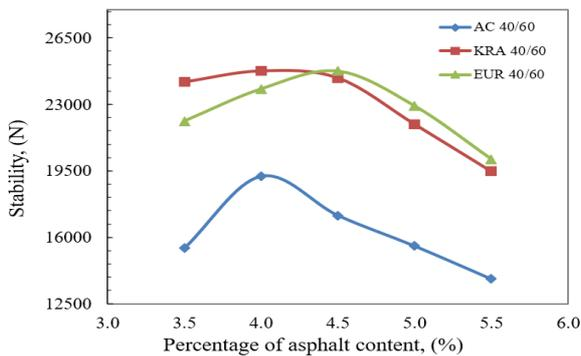
Fig. 8. Variations of stability with asphalt content percentage.
