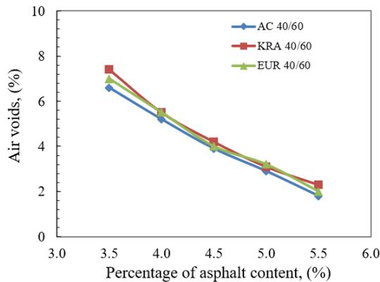
Fig. 7. Variations of air voids with asphalt content percentage.
