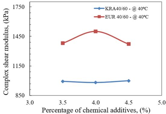
Fig. 6. Variations of complex shear modulus viscous portion with chemical additives percentage.
