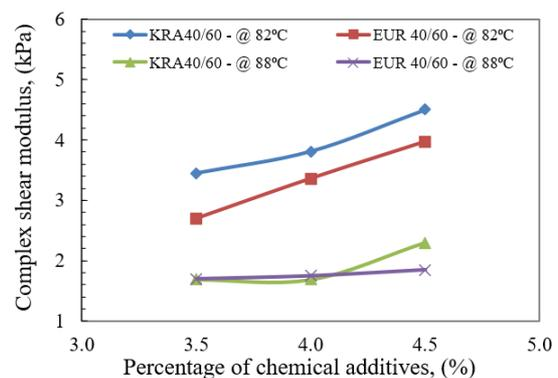
Fig. 5. Variations of complex shear modulus elastic portion with chemical additive percentage after changing weight percent.
