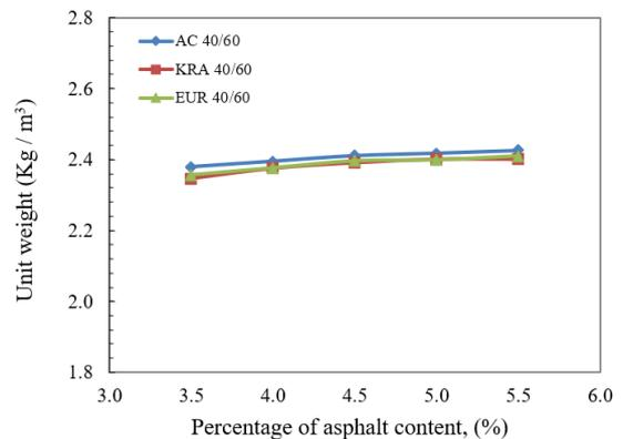
Fig. 10. Variations of unit weight with asphalt content.
