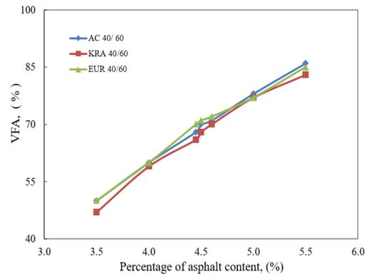
Fig. 9. Variations of percent voids filled with asphalt content.
