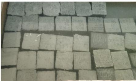
Fig. 4. Curing of concrete specimens.
