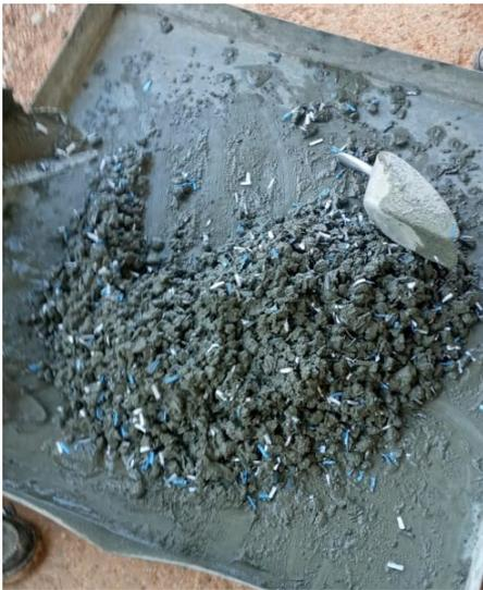
Fig. 3. Mixing of concrete with added SUSFM fibers.
