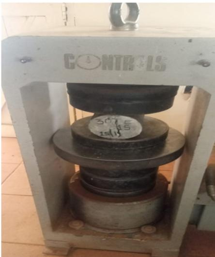
Fig. 5. Concrete split tensile strength testing.
