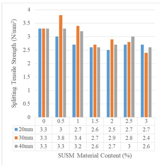
Fig. 8. Split tensile strength of concrete with different contents and lengths of SUSFM fibers.
