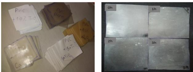
Fig. 1. Samples before and after electric aging.
