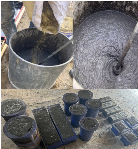
Fig. 4. Casting SIFCON using the gradual mix method.
