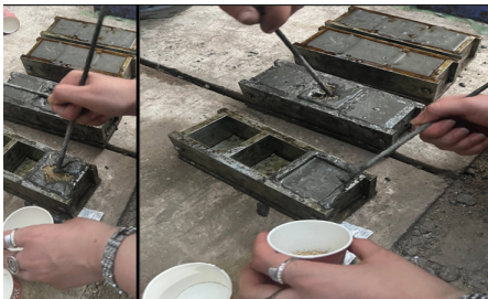
Fig. 3. Casting SIFCON using the multi-layer method.
